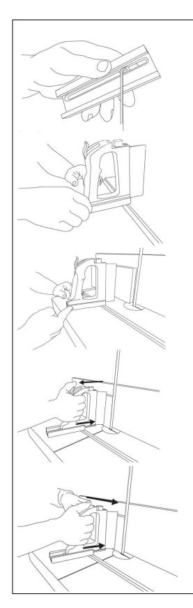
Diagram 1: Adjust position of Miter Cam in GuidePRO Base
