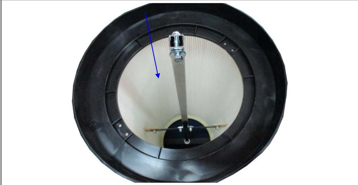
Step Thirty Six: Assemble the canister filter to the dust chute. Tighten the band clamp and adjust the tightness accordingly to ensure the canister filter is tightly fitted onto the dust chute.
