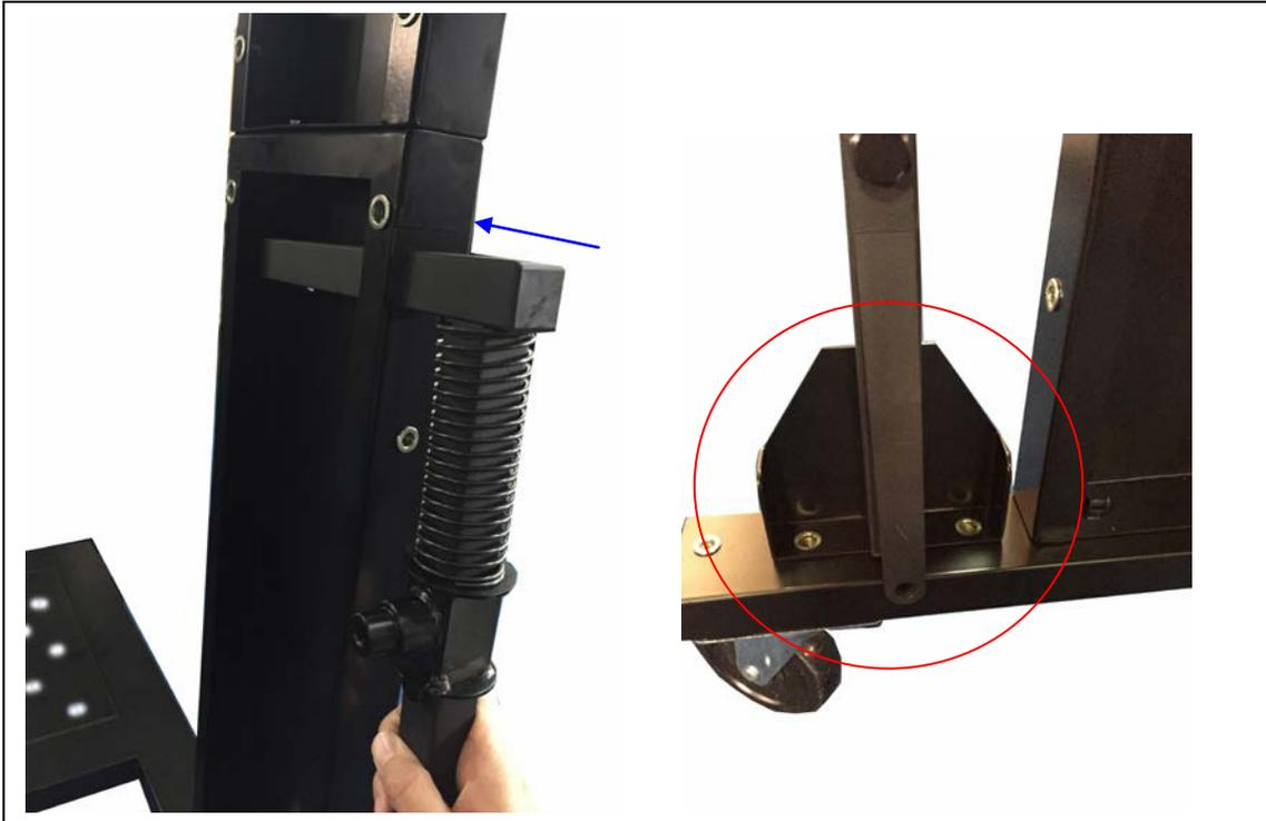
Step Eleven: Secure the foot pedal support to the lower upright support panel using (4) 5/16"×1/2" carriage bolts, (4) 5/16"×OD18\*2t flat washers and (4) 5/16" hex nuts. Then secure the foot pedal bar to this support using (4) 5/16"×1-3/4" hex bolts, (8)5/16"×OD18\*2t flat washers and (4) 5/16" hex nuts. Follow the same steps for the opposite side.
