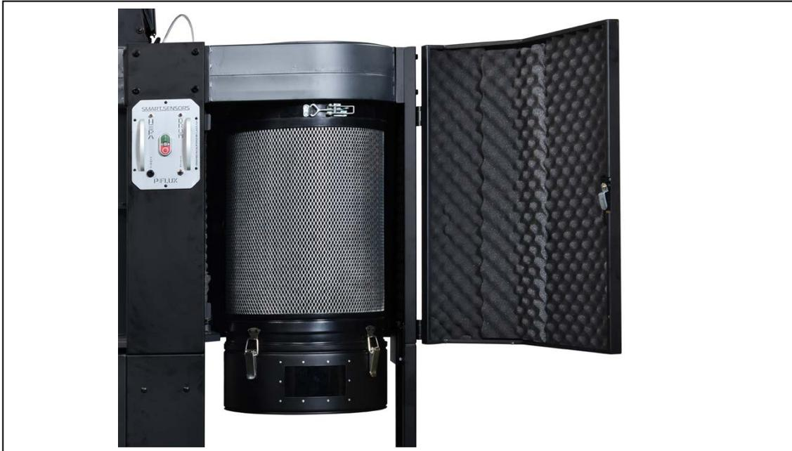
2. While the cyclone is collecting the dust from inside the canister end cap; use compressed air and an air gun and blow the outer surface of the canister.
