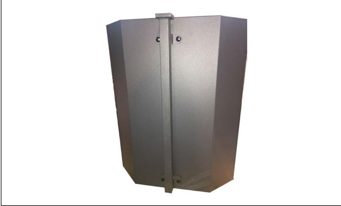
Step Forty Seven: Take the one of the cover plates, (2) 1/4" x 1/2" carriage bolts, (2) 1/4" x OD19\*2t flat washers and (2) 1/4" hex nuts and secure the cover plate to the opening on the top of the drum. For the bottom holes do the same, but first use foam tape to cover the square opening before bolting on the cover plate.
