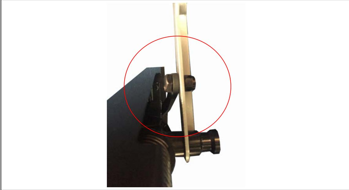
Step Twenty Five: Apply foam tape to the cone flange before attaching the drum lid. Secure the Octagon drum lid to the cyclone funnel using (8) 5/16"×3/4" hex bolts, (16) 5/16"×OD18×2t flat washers and (8) 5/16" hex nuts. Make sure to first attach all the bolts on before tightening the bolts. **The lid will turn when the bolts have not been tightened for alignment.** Failure to do will result in the drum lid not being able to align with the drum.
