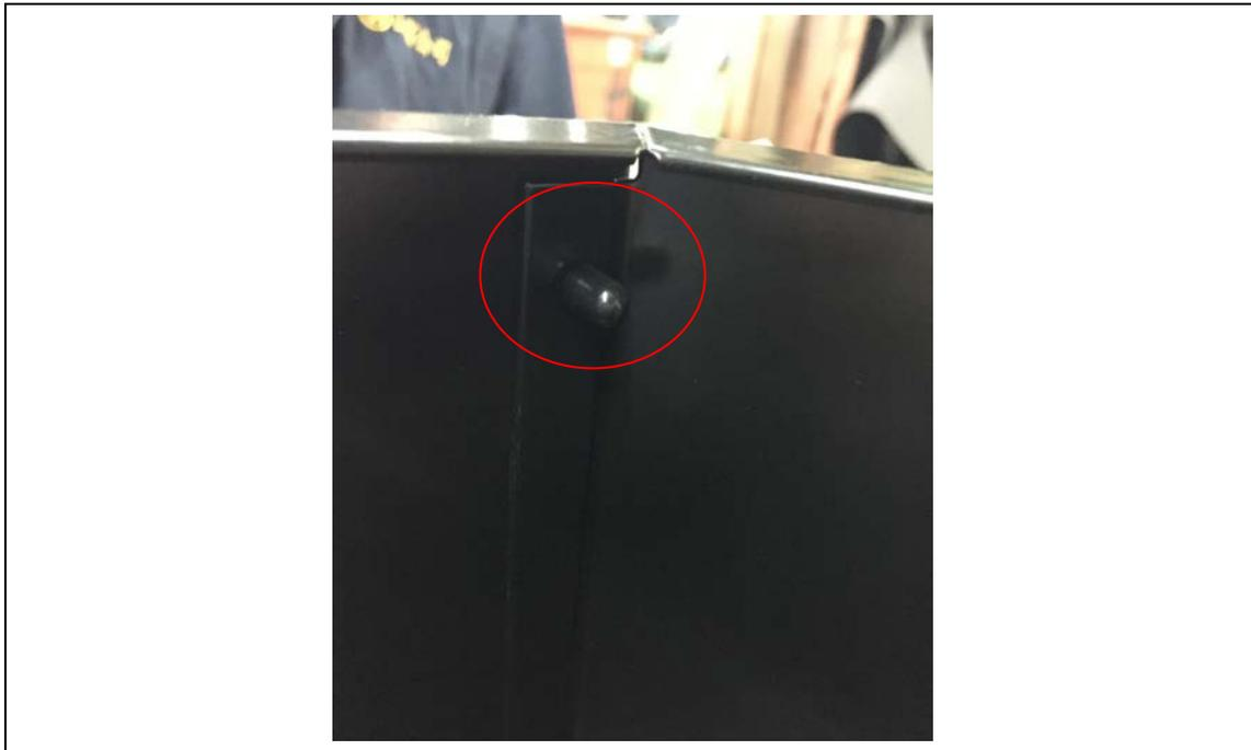
Step Thirty Five: Once completing the assembly, apply silicone to the inside of the drum including the base to seal and prevent air leakages.
