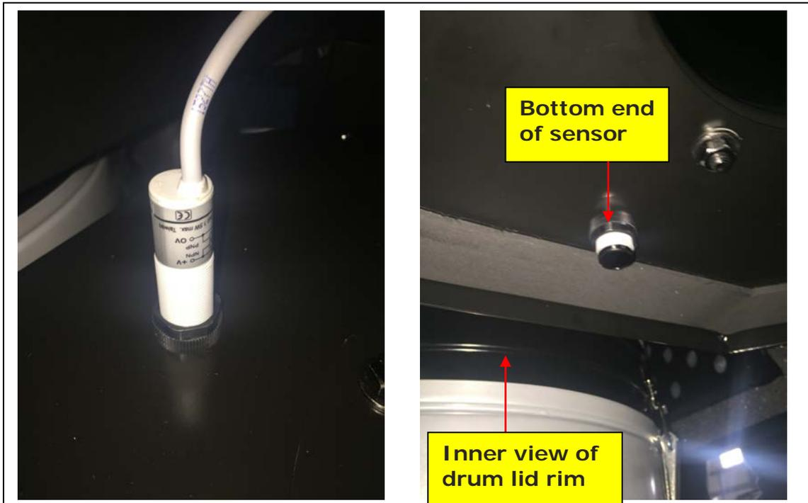
Step Twenty Seven: To adjust the distance of the sensor to detect the dust waste level use the white plastic pin that was provided in the hardware box.
