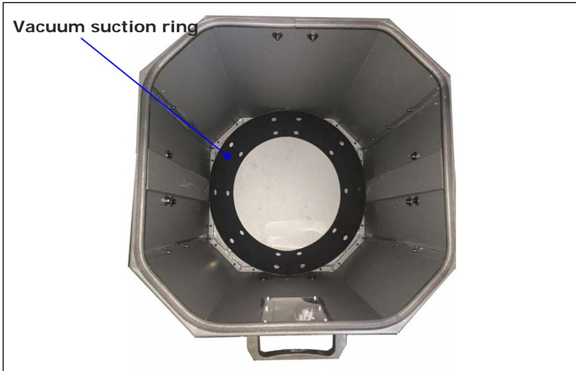
Step Thirty Nine: Insert the plastic bag inside the Octagon drum. Open and spread out the plastic bag to the corners and edges
