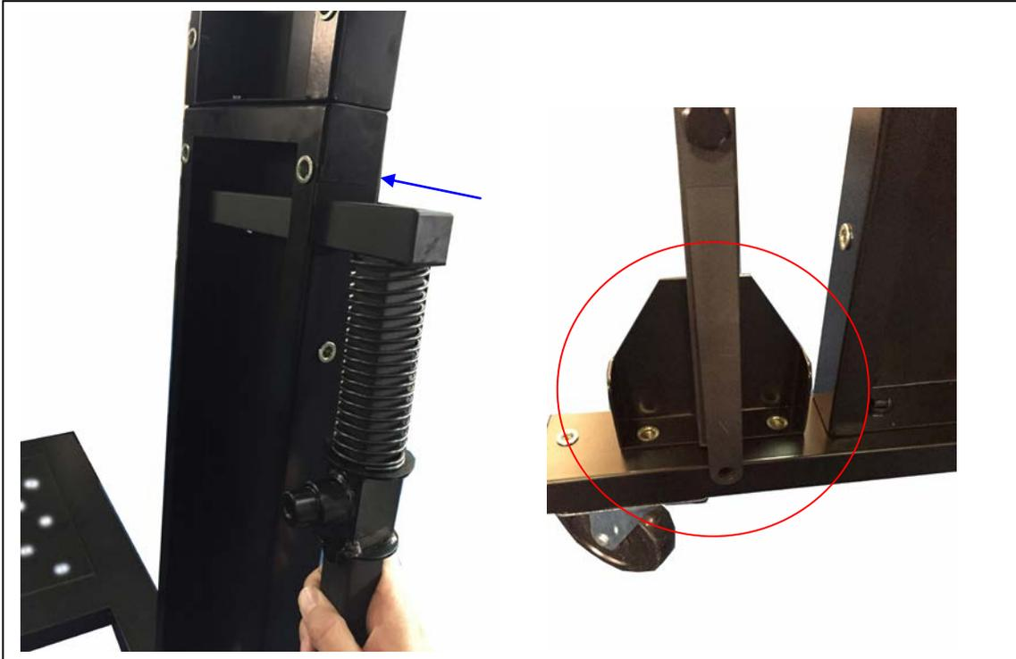
Step Seventeen: Secure the foot peddle support to the lower upright support panel using (4) 5/16"×1/2" carriage bolts, (4) 5/16"×OD18\*2t flat washers and (4) 5/16" hex nuts. Then secure the foot peddle bar to this support using (4) 5/16"×1-3/4" hex bolts, (8)5/16"×OD18\*2t flat washers and (4) 5/16" hex nuts. Follow the same steps for the opposite side.
