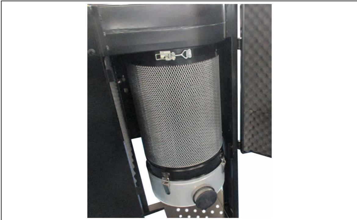
2. While the cyclone is collecting the dust from inside the canister end cap; use compressed air and an air gun and blow the outer surface of the canister.
