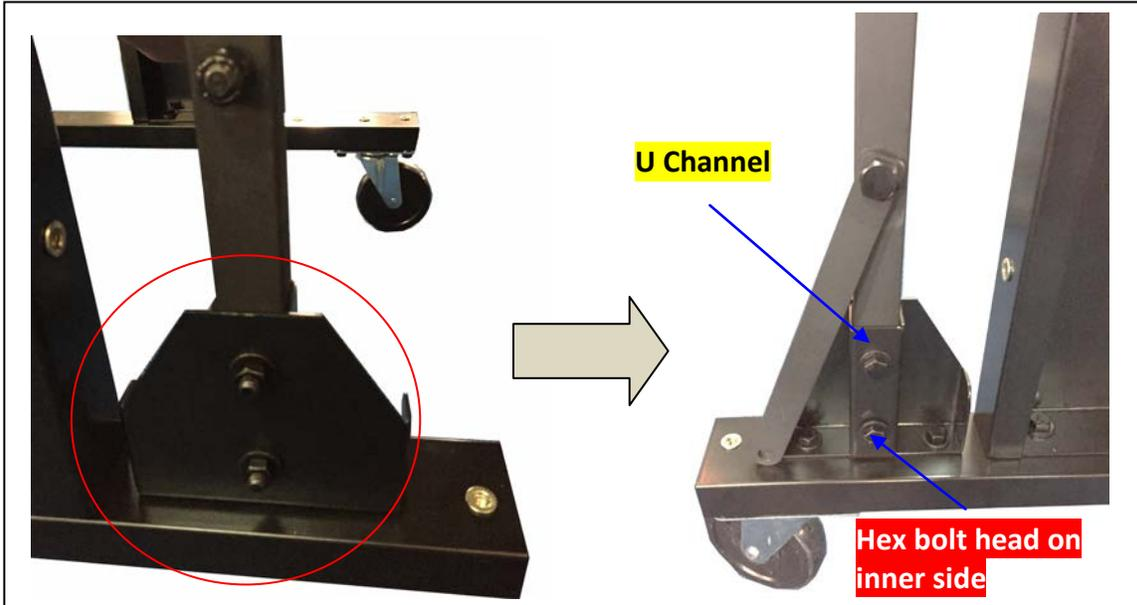
Step Nineteen: Attach the cover plate over the foot peddle assembly. Secure using (6) 1/4" x 3/4" hex bolts and (6) 1/4" x OD19\*2t flat washers. Follow the same steps for the opposite side.
