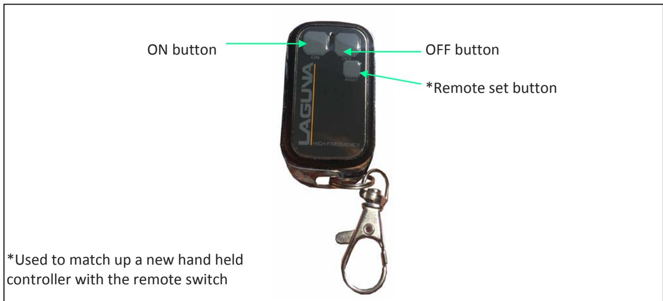
\*Used to match up a new hand held controller with the remote switch
