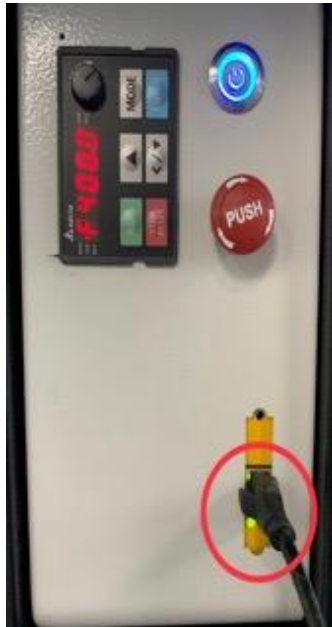
Figure 7: Push the power button and plug in Ethernet connector into PC and controller
