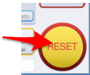
Figure 54: Reset to disable spindle relay
