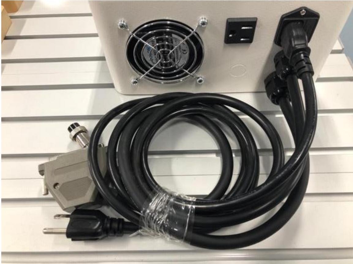
Figure 4: Cable summary out of control box
