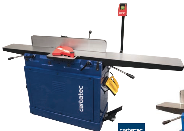
CARBATEC 8" Long Bed Helical Cutterhead Jointer with Parallelogram Tables Part No. JN-X200C ▪ 1100 W (1 ½ HP) induction motor ▪ Integral mobile base ▪ Parallelogram bed adjustment ▪ 4" Dust port ▪ Max. cutting width 200 mm Also available with straight blade.
