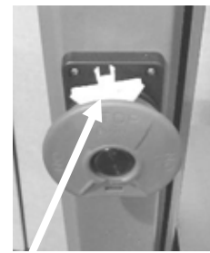
Start/stop with safety removed
