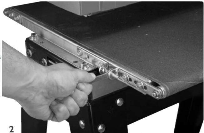
2 Loosen the conveyor take-up screws to relieve belt tension and slide the drive roller fully inward.
