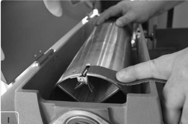
Start on the left (outboard) side of the drum. Pinch or squeeze the clip lever and insert the tapered end of the paper through the slot and into the fastener so that it uses most of the width of the slot. Release the clip lever to securely hold the end in the fastener.
