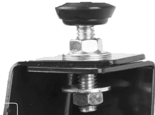
Thread a hex nut onto each of the leveling feet attach a leveling foot to the bottom of each leg with the hardware order as shown (not required if installing optional caster set #98-0130).
