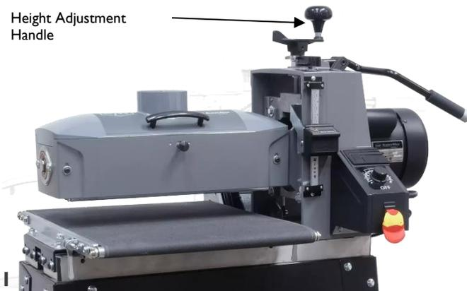
1 Raise the drum carriage to its highest position using the height adjustment handle. Turn off power source to machine. Unplug main drive motor from receptacle (in gear motor assembly).
