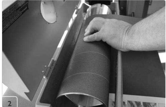
Wind the wrap around the drum, being careful not to overlap the windings. The tapered cut of the wrap end should follow the edge of the drum.
