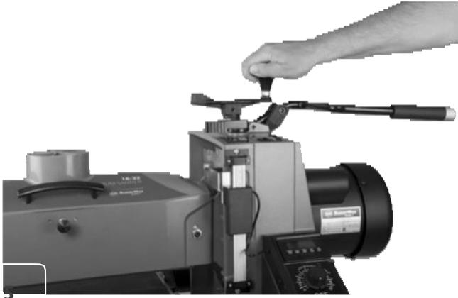
Raise the head of the sander by rotating the height adjustment handle up exactly one full turn.
