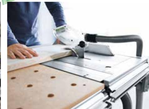
A range of system accessories allow you to upgrade to a complete sawing station with minimal effort. Even cross cutting sections up to 803 mm on both the floor and set version.
