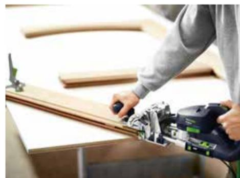
A clever and unique portable mortise and tenon machine that lets you join anything - from narrow workpieces to large panels.
