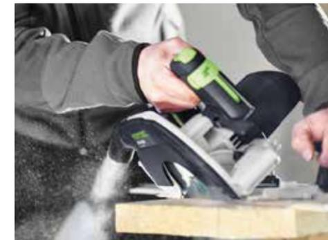
When sawing with a Guide Rail the cutting edge follows the scribe mark edge exactly for precise results even when mitre cutting.
