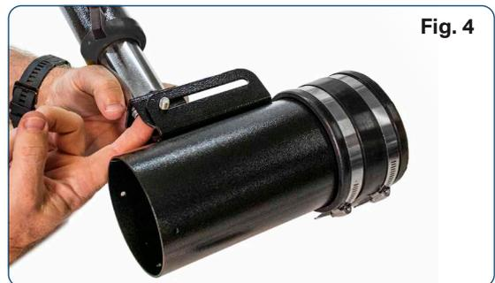
5. Attach your selected dust hood and hose with the supplied clamp, or any standard 4" hose clamp.
