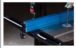
The aluminium fence is incredibly strong, straight, and built to last for years. The face and top edge of the fence contain T-slots for adding stops, resaw guides, and more.
