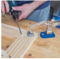
Bench Clamp keeps pieces perfectly aligned to create tight-fitting joints.
