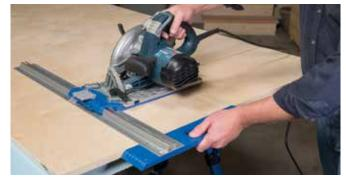
Straight cuts are easy thanks to an oversized edge guide with a hand-hold that provides control through the entire cut by following the edge of your sheet.
