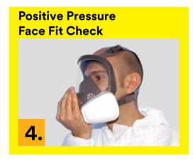
Place the palm of your hand over the exhalation valvecover and exhale gently. If the facepiece bulges slightly and no air leaks are detected between the face and the facepiece, a proper seal has been obtained.
