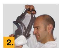
Pull the face respirator down over the head placing the nose and chin in the nose cup/chin area. Then press the facepiece firmly and evenly against the face. Pull head harness to back of head.
