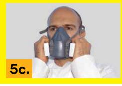
With Solid-top Particulate Filters: Squeeze filter covers together using the palms of your hands and fingers to restrict airflow. Inhale gently. The facepiece should collapse slightly.
