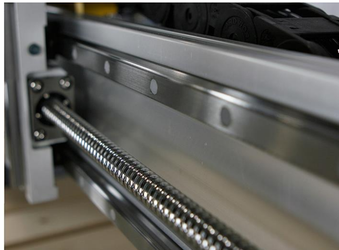
Figure 81: Weekly (best case daily) cleaning and application of light oil externally to screws and rails with cloth and light oil.
