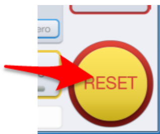
Figure 67: Reset to disable spindle relay
