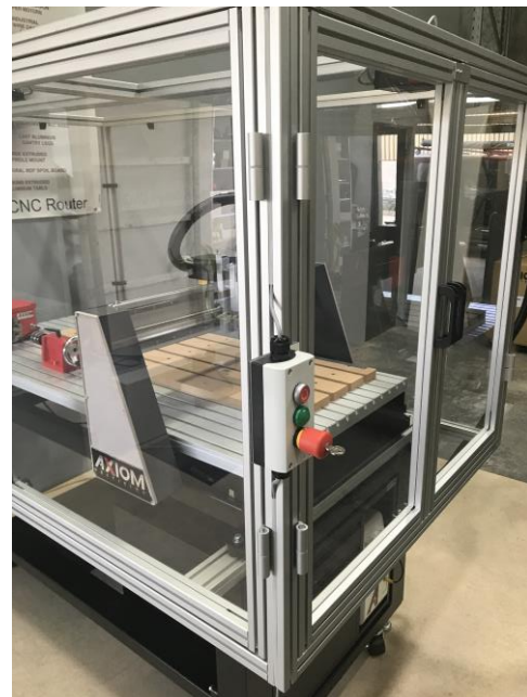
Figure 36 Safety Enclosure Main Controller
