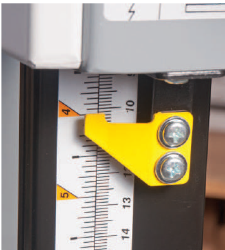
Upper blade guide height scale and pointer
