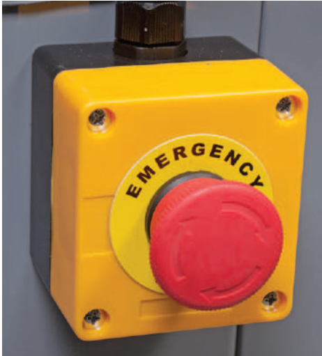
Emergency stop, press to stop the bandsaw
