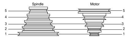
Figure 20 - Spindle Speed Adjustment
