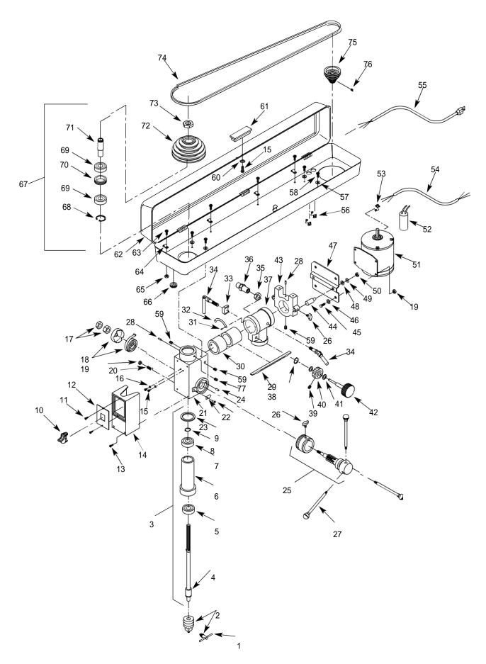
Figure 25 - Replacement Parts Illustration for Head
