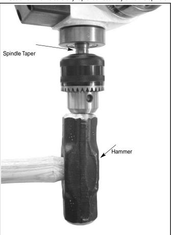
Figure 12 - Secure Chuck onto Spindle
