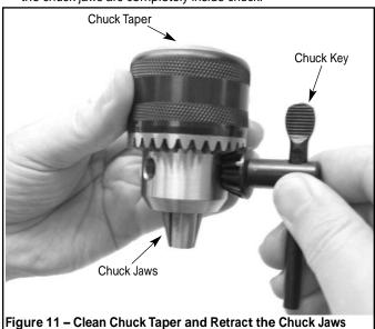
Push chuck over spindle taper and twist chuck slightly to release air trapped in taper.
