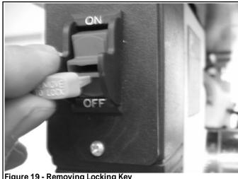
Figure 19 - Removing Locking Key
