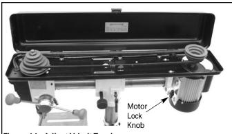
Figure 14 - Adjust V-belt Tension
