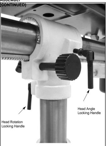
Figure 10 - Secure Head Assembly
