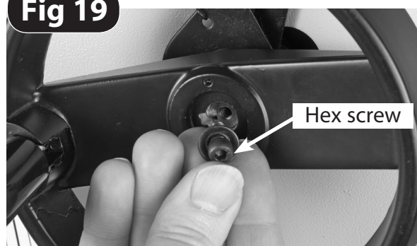
Insert the hand wheel over the shaft for the tilt mechanism
