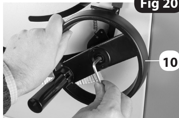
Secure the hand wheel in place using a Hex screw and washer then tighten using the supplied Hex key
