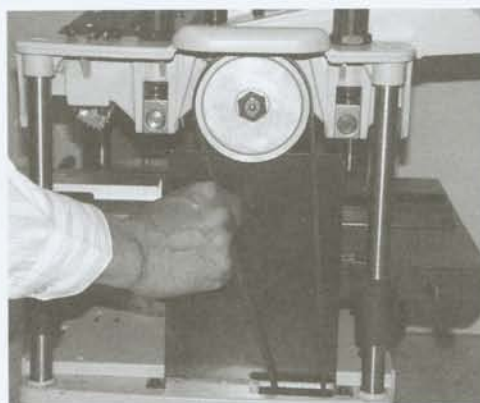
Rotate the cutterhead by moving the belt by hand.
