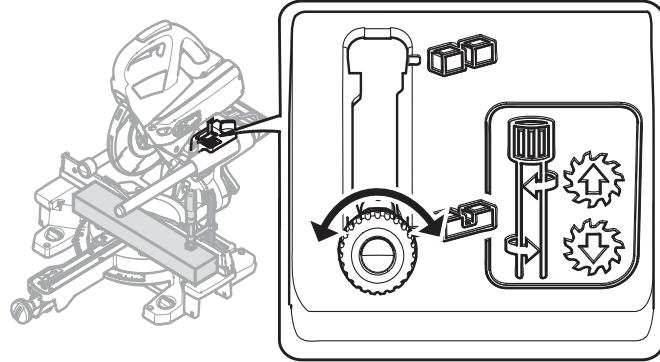
**i** Only turn down the lever for the groove depth limit **[1-4]** if the saw unit is in the upper position (= working position).
