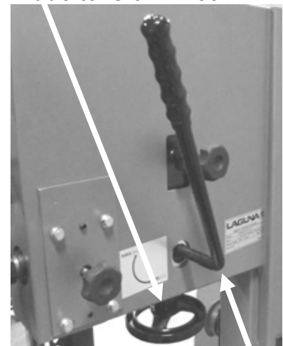
Quick action blade tension lever (activated)
