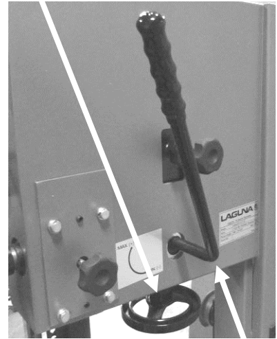
Quick action blade tension lever (activated)
