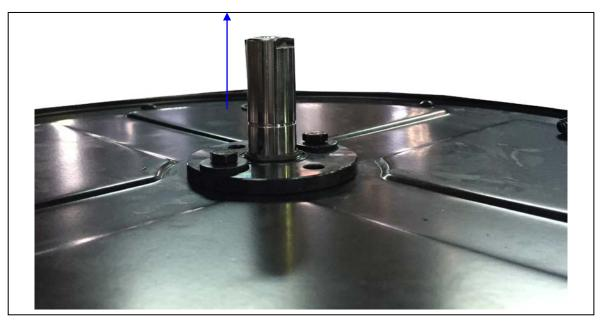
Step Forty: Secure and tighten the (1) 5/16"\*3/4" and (1) 5/16"\*OD23\*2t flat washer on the rotation shaft base.
