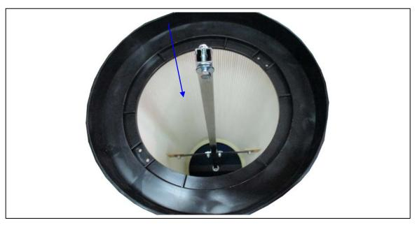
Step Thirty Six: Assemble the canister filter to the dust chute. Tighten the band clamp and adjust the tightness accordingly to ensure the canister filter is tightly fitted onto the dust chute.
