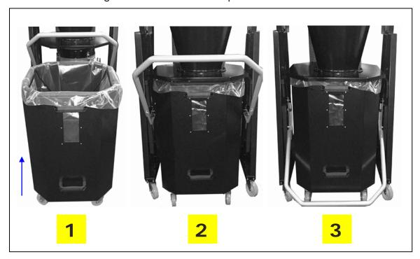
Step Thirty One: Make sure when aligning the drum that both the left and right side lift plates are over the topping on the foot peddle bar assembly before lifting the foot peddle bar up. When not aligned, the drum will not be fully sealed and will interfere with the air flow.
