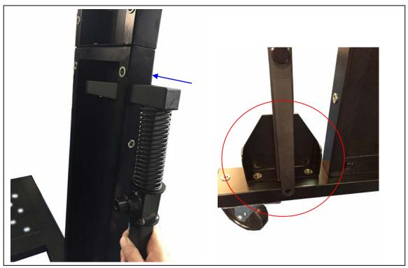
Step Eleven: Secure the foot pedal support to the lower upright support panel using (4) 5/16"\*1/2" carriage bolts, (4) 5/16"\*OD18\*2t flat washers and (4) 5/16" hex nuts. Then secure the foot pedal bar to this support using (4) 5/16"\*1-3/4" hex bolts, (8)5/16"\*OD18\*2t flat washers and (4) 5/16" hex nuts. Follow the same steps for the opposite side.
