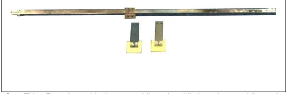
Step Thirty Four: Assemble the two paddle and paddle branch assemblies to the rotation shaft using (4) 1/4"\*5/8" hex bolts, (8) 1/4"\*OD13\*1t flat washers and (4) 1/4" hex nuts.
