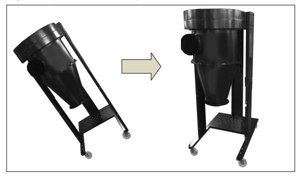
Step Nine: Secure the lower triangular support plate to the base using (4) 5/16"\*3/4" hex bolts and (4) 5/16"\*OD18\*2t flat washers. Follow the same steps for the opposite side.
