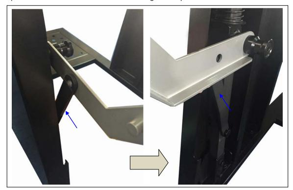
Step Seventeen: Secure the movable supporting brace on the foot pedal bar with the octagon foot pedal using(2) 3/8"\*46mm hex bolts. Make sure the bolt head is on the inside of the octagon handle. Adjust the tightness of this bolt accordingly. If this bolt is too tight, the Octagon foot pedal will not work smoothly. When too loose it will not pick up the Octagon drum.
