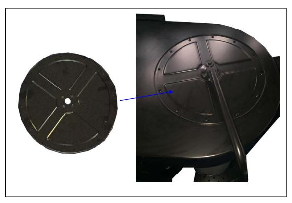
Step Thirty Eight: From the bottom of the canister filter, push the rotation shaft through the hole in the middle of the canister cover plate.
