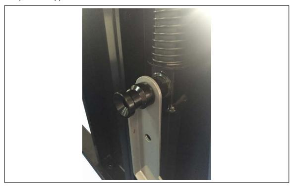
Step Fifteen: Secure the topping with (2) M8\*30mm hex bolts
