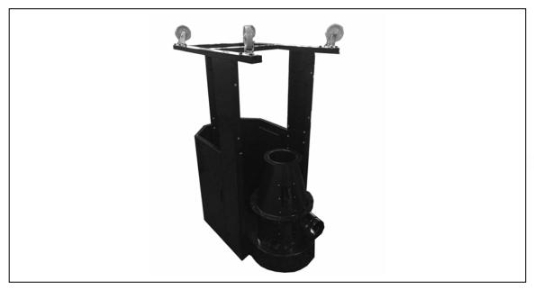
Step Seven: Secure the (3) upright support reinforcement plates using (12) 5/16"\*3/4" hex bolts and (12) 5/16"\*OD18\*2t flat washers.
