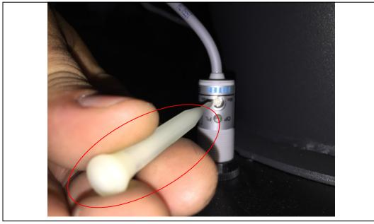
Step Twenty Five: Using the white plastic pin, insert the sharp point into the top end of the proximity sensor that is on top of the drum lid. You will find a small hole to on top where you can turn clockwise or anti-clockwise.
