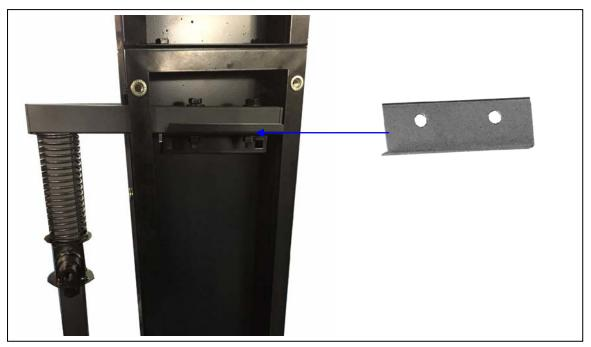
Step Fifteen: Secure the base of the foot pedal bar to the triangular support plate by holding the lower support plate vertically up against the foot pedal bar and securing the U channel provided onto the foot pedal bar using (2)5/16\*\*1-3/4\* hex bolts, (4) 5/16\*\*OD18\*2t flat washers and (2) 5/16\* hex nuts from the inside out. Follow the same steps for the opposite side.
