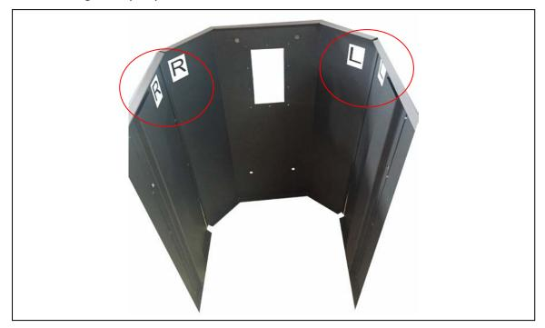
Step Twenty Nine: Both the left and right side lift panels have three bolt holes on them. Take the matching side plate and secure to the outside of the panel. (Photo shown is the inside of the panel) using (6) 1/4"\*1/2" carriage bolts, (6) 1/4"\*OD19\*2t flat washers and (6) 1/4" hex nuts.
