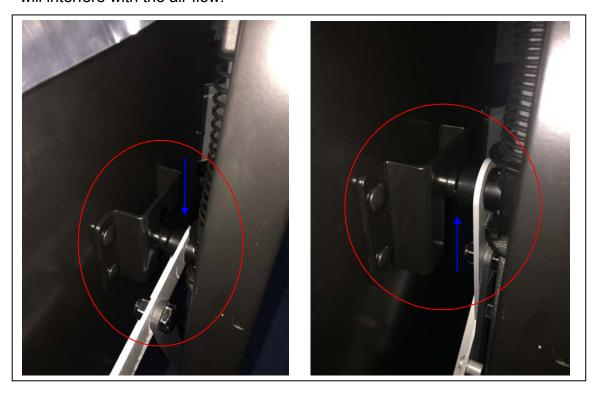
Step Thirty Nine: Remove the control panel by loosening the six bolts holding it to the panel. Secure the two handles to the control panel using (4) M4\*6mm philip hd bolts.
