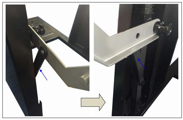
Step Twenty One: Secure the movable supporting brace on the foot peddle bar with the octagon foot peddle using (2) 3/8"\*21mm hex bolts. Make sure the bolt head is on the inside of the octagon foot peddle. Adjust the tightness of this bolt accordingly. If this bolt is too tight, the Octagon foot peddle will not work smoothly. When too loose it will not pick up the Octagon drum.
