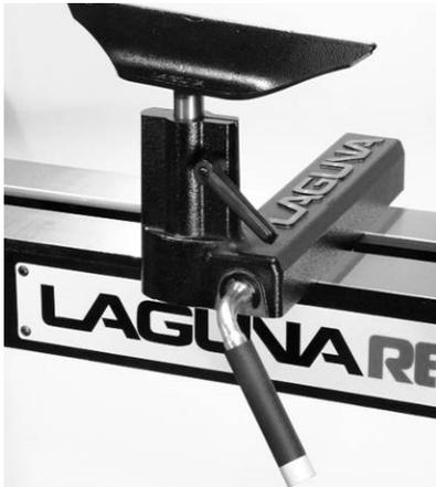
Tool rest assembled to the bed
