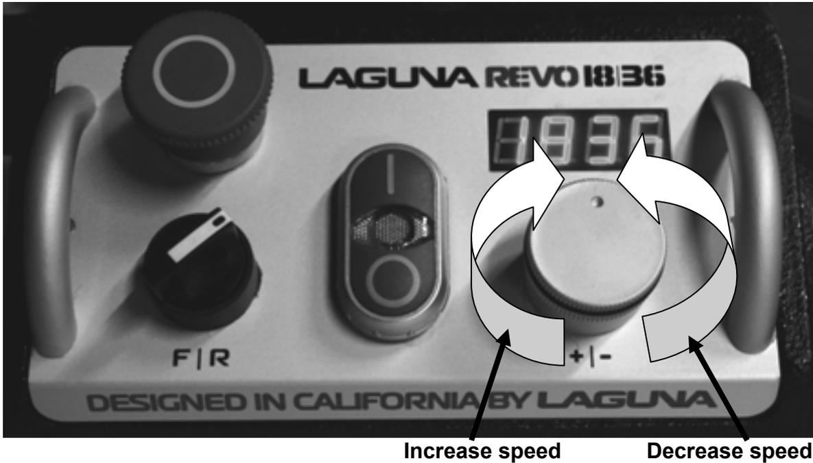
The Variable speed adjustment knob adjusts the spindle speed. Turns clockwise to increase the speed, turns counter-clockwise to decrease the speed
