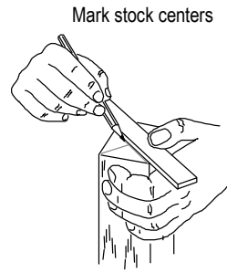
For hardwoods - drill centers and saw diagonals for spur center
