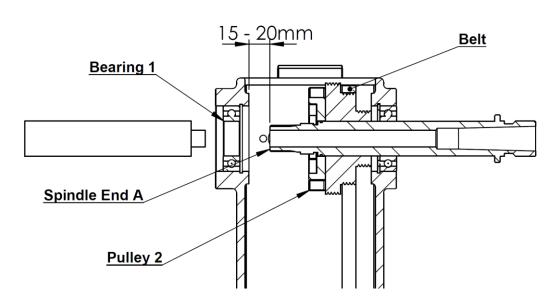
7. Remove the old belt and place the new belt over the **Spindle End A** and on to **Pulley 2**.
