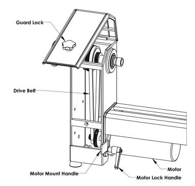
6. Tension the belt by pressing down on the Motor Mount Handle. Pressing down with 2 fingers or the thumb will provide adequate pressure. Slightly higher pressure may be required for larger work.
