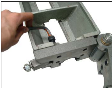
Fig 4. Attaching part 9009 to bed View from underneath
