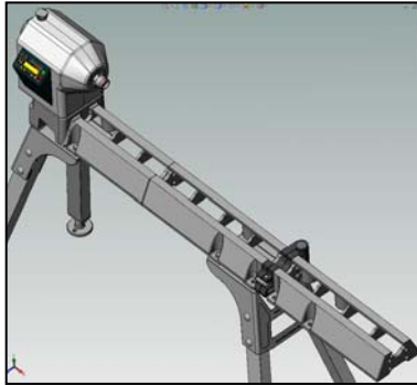
Fig. 6 Use with DVRXP / 1624 lathe and Headstock
