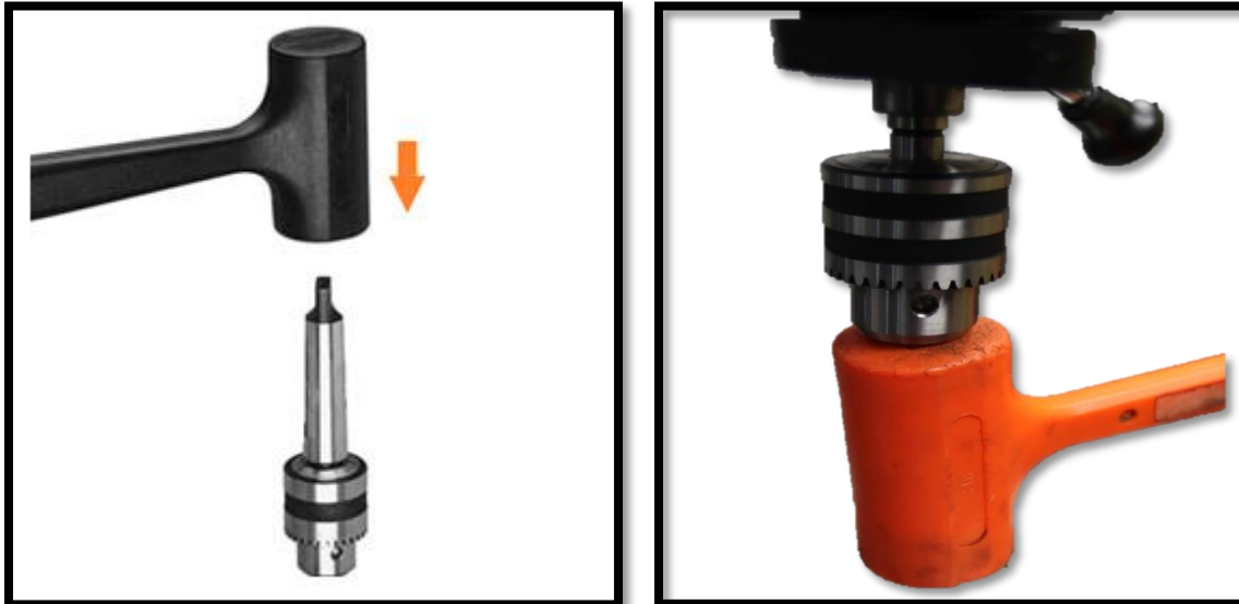
Figure 9 - Seating arbor into drill chuck (left) & Seating arbor and chuck into spindle (right)
