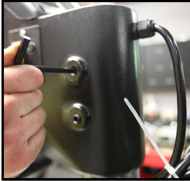
Figure 5 - Mounting the headstock
