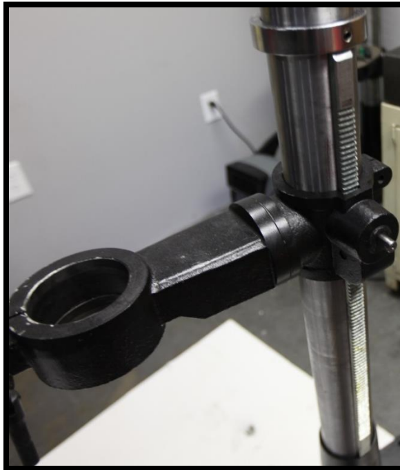
Figure 4 - Mounting the table bracket and rack 2/2
