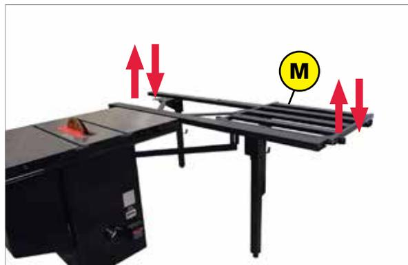
Check the rear bearing by lifting up and then pushing down on the rear of the sliding table.
