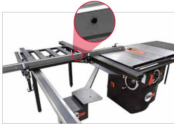
Slide the crosscut fence ruler until the right edge of the flip stop indicates the measurement of the cut piece of wood. Re-tighten the hex head bolt.
