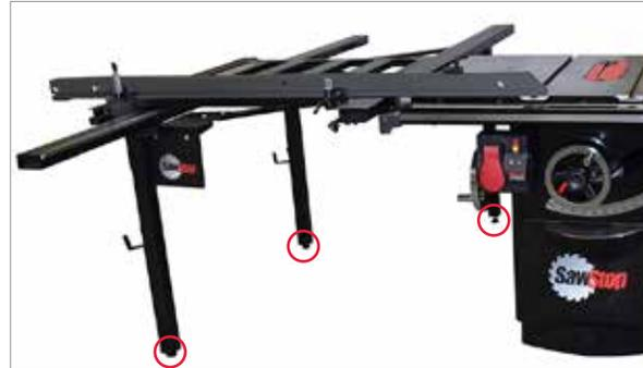
**4** Use a 13mm wrench to tighten the hex head bolt closest to the front of the saw and to loosen the hex head bolt closest to the rear of the saw.
