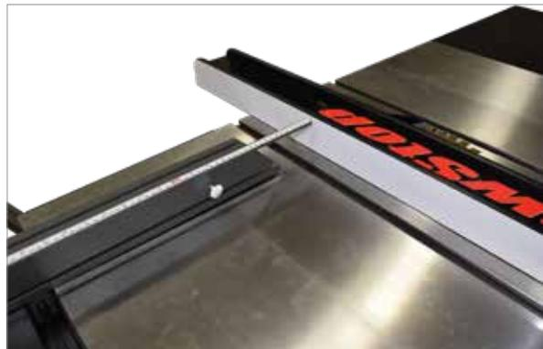
If there is no variation along the whole distance of the straightedge or ruler, skip adjustment steps 7-12 below. If any variation between the end of the crosscut fence ruler and the straightedge or rip fence is observed, proceed to step 7 below.
