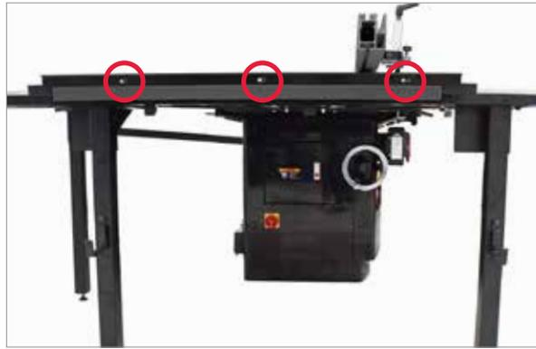
**8** Check the miter angle ruler. If the reading is not 0 degrees, loosen the hex head bolt near the middle of the inside edge of the angle guide rail and adjust the position of the miter angle ruler to read 0 degrees. Re-tighten the hex head bolt.
