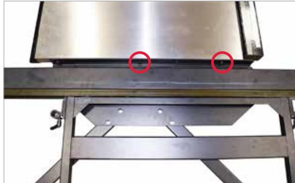
**For PCS only:** Use a 13mm wrench to slightly loosen the front three hex head bolts attaching the mounting bracket to the extension wing or saw table.
