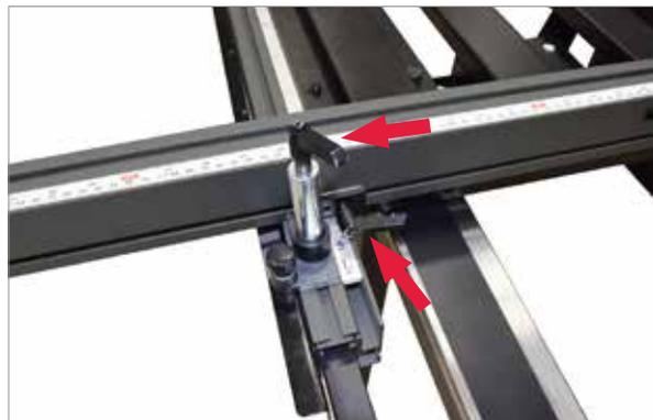
**7** Recheck the alignment between the crosscut fence and the blade. If necessary, use a 10mm wrench to loosen the three hex head bolts securing the miter detent pin positioning bracket to the guide rail and use the clearance provided by the elongated slots to realign the 90 degree hole with the miter detent pin in the fence lock assembly. Re-tighten the three hex head bolts.
