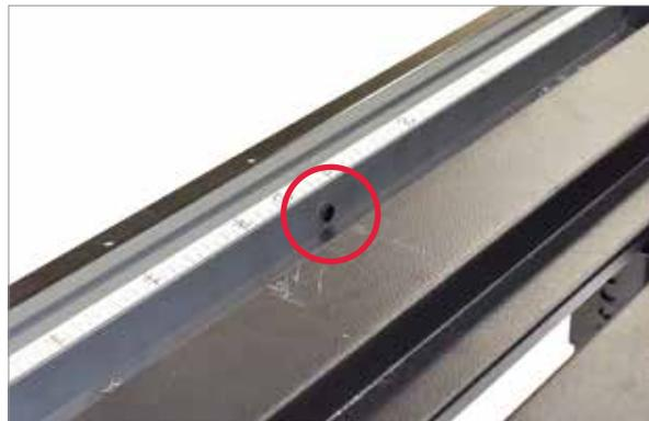
**9** The miter detent pin positioning bracket has five holes in the top, which correspond to 90, 15, 22.5, 30, and 45 degrees for the crosscut fence. The holes can be used to quickly align the crosscut fence for miter cuts without having to use the miter angle ruler.
