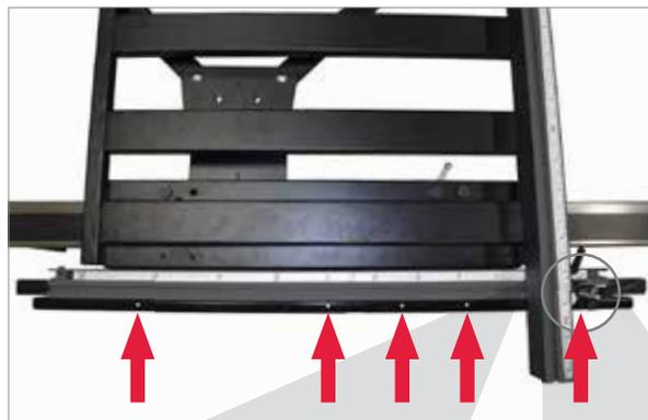
When aligning the fence with the desired marking on the miter angle ruler, read markings on the side of the fence that faces away from the operator.
