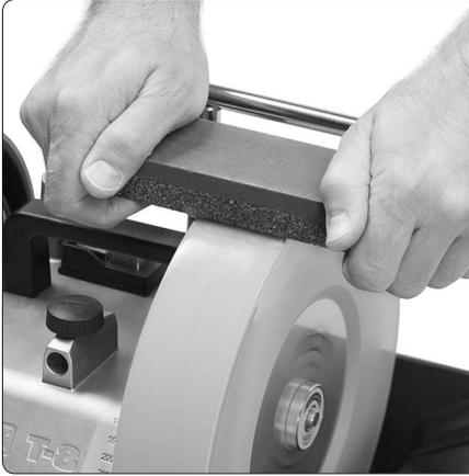
*Made of silicon carbide, one side with a very fine grit and the other side with a coarse grit.*
