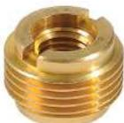
Made of brass with knife-edge external threads to securely thread into a 1/2" pre-drilled hole, internally threaded to accept 5/16" x 18TPI bolts. Insert requires a 3/8" pre-drilled hole.
