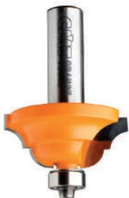
A favourite traditional profile for moulding, architraves etc. A Classical Roman Ogee profile, with the addition of a horizontal bead at the mid transition point. Ball bearing guided.
