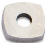
This Robert Sorby HSS external shear scraper cutter is set to an angle of 45°, to get a good shear cut. This type of cut is less aggressive and leaves a finish that requires little to no sanding. It is an excellent choice for external work.
