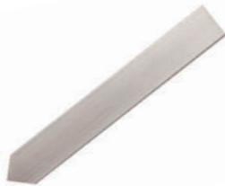
This Robert Sorby double ended cutter is spring loaded into a chatter tool, giving a unique decorative pattern to end grain only. Alternate patterns are achieved by adjusting cutter lengths, Changing cutter shape, Altering lathe speed, Traverse or stationary cuts, and Cuts on, above or below centre.
