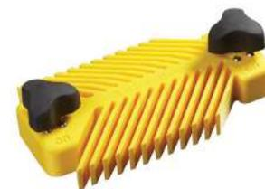
Low profile and double sided, this is the most versatile Featherboard from Magswitch. Works to improve your cutting results on either side of the blade. Also designed to work on any cast-iron fence to hold down your work so you don't have to. Great for small tables! Features two 20mm Magswitches. No mitre slot limitation. Dimensions: 175 long x 100 wide x 26mm thick.
