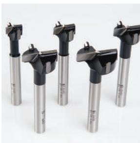
Used for drilling blind holes into solid wood, wood composites and plastic laminated materials for concealed hinges, creating holes or recesses for hardware or accessories or simply to remove waste in wood turning. With the cutting tips being Tungsten Carbide, the user will get and life before sharpening is required, therefore extending the life of the bit. The sharp
