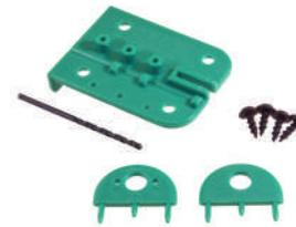
These splitters are green, identifying them for thin kerf blades, 3.0mm to 3.2mm. Used by woodworkers around the world, the MicroJig Splitters are positioned so one is in the same plane as one side of the blade, and the other is in the same plane as the other side of the blade. The splitters are tapered, so will not bind on the timber as it is being cut. When cutting some timber,
