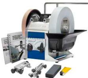
Sharp tools in the workshop or jobsite make working so much easier and safer, a sharp blade takes less effort to push through the job, whether that is dovetails, mortices or woodturning projects. The slow rotation in the water bath gives a cool grind, so no heat is generated in to steel that could alter its composition or ability to keep an edge.
