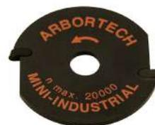
The safe way to do fine and detailed carving work. This is a great choice for shaping, cutting, trenching or planing on material both with or against the grain. The blade is designed with a chip limiter which prevents cuts being too deep and prevents grabbing and kickback. The teeth are Tungsten Carbide tipped, so can be resharpened using a fine diamond abrasive, but are not replaceable. This blade is 2" in diameter. Kit includes: 1 x Mini Industrial Blade; 1 x Brass Reducing Washer.
