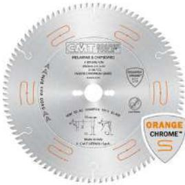
Ideal for cutting ply, and melamine, this blade features CMT's general purpose chrome coating and laser cut noise reduction slots. The coating protects the blade from overheating, prevents corrosion and rust, minimises resin build-ups, improves chip ejection and improves performance and cutting life. The noise reduction slots are filled with orange polyurethane that reduces vibration and noise making this blade cut smoother, quieter and cleaner.
