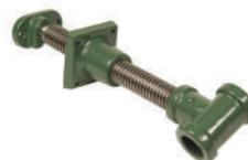
This vice screw is specifically for the type of 'L' shaped shoulder vice used on Scandinavian style benches. It has a 1-1/8" (29mm) diameter screw with single lead Acme threads. The threaded guide is morticed into the vice shoulder, while the end guide attaches to the vice jaw. 9" (229mm) clamping capacity, 13" (330mm) overall.
