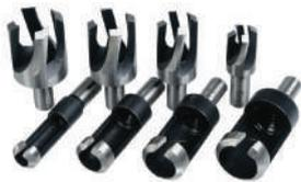
Set includes two types of plug cutters: barrel plug cutters and plug counter-bores. Diameters include 1/4", 3/8", 1/2" and 5/8". Plug lengths vary from 9mm to 18mm.
