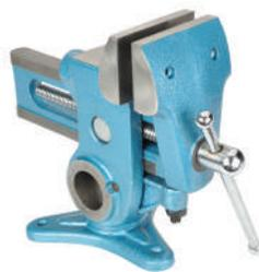
The Parrot vice incorporates a unique tightening cam that lets it pivot freely through 360 degrees until you tighten the jaws firmly, locking the vice in place. This allows you to back off the clamp screw just enough to rotate the vice for access to any part of a workpiece without releasing it from the jaws. Additionally, the vice can be
