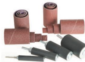
This is an economical set of sanding drums in standard size spindles, 13mm (1/2"), 19mm (3/4"), 25mm (1") and 38mm (1-1/2"). All spindles are 63mm (2-1/2") long. Two 80 and 120 grit sleeves are included for each drum. Generally used in a drill press or lathe to eliminate the need for an oscillating spindle sander.
