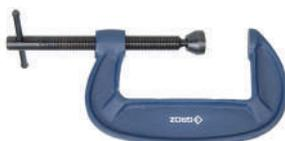
Extra high quality G clamps. The body is made of malleable cast iron and screw and pin are made from high quality steel for long life. Indispensable for any workshop! Throat 60mm, Width 100mm.
