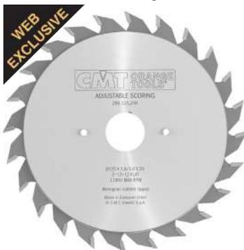
Used on a vertical or horizontal panel saw to prevent chip out on laminate materials. Smaller in size than the main blade, it spins in the opposite direction to that of the main blade, and cut a channel slightly wider than the main blade, but not wide enough to be noticeable when edge tape is applied. Shims placed between the two split blades to match the main blade.
