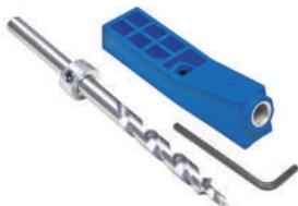
The Kreg Jig Mini is good for very specific applications where the smallest jig possible is required. The simplistic design includes the hardened-steel drill guide of the other jigs, but does not include a reference fence, so material thickness adjustments must be made manually. The fenceless design allows you to make precise angle and stock depth adjustments as needed, making the Mini the most positionable Kreg Jig available. The relief hole allows waste
