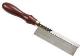
Japanese Razor Saw 120mm blade 0.2mm kerf and 48TPI. Suitable for cutting dovetails or other cuts where precision is essential.
