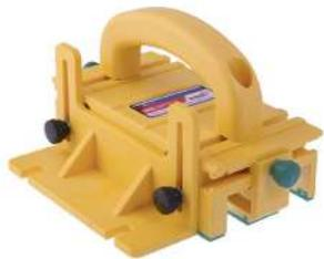
The GR-100 GRR-RIPPER grips the workpiece securely and safely. Featuring two fixed outer feet, and a third adjustable wider inner foot moves so it can be positioned either side of the blade depending on the width of cut. The inner foot that goes towards the fence is 6.35mm (1/4"), so it can cut stock down to this width. Even catering for bevel cuts safely, keeping
