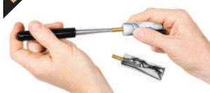
This helpful pen tube insertion tool is versatile enough to work on any pen kit - from Slimline through the Majestic. Now one insertion tool is all you need. Accepts and inserts tubes from 7mm through 37/64.
