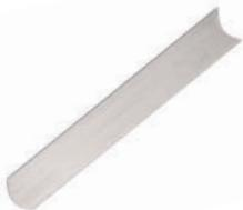
This Robert Sorby double ended cutter is spring loaded into a chatter tool, giving a unique decorative pattern to end grain only. Alternate patterns are achieved by Adjusting cutter lengths, Changing cutter shape, Altering lathe speed, Traverse or stationary cuts, and Cuts on, above or below centre.
