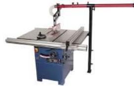
This suva guard is the ideal solution for providing safety and dust control when operating a table saw. When connected to a dust collection system, the suva guard captures dust thrown up by your table saw blade. It can be used on any saw with an extension table. It is simple to install and swings out of the way when not in use - a
