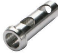
The RSB-SOV-C13 has the widest aperture for tools made from round section at 1/2" and is perfectly aligned to take 3/8" bowl gouges and fingernail bowl gouges, the 1/2" spindle gouge, fingernail spindle gouge and the long and strong spindle gouge as well as the Turnmaster. The Spiralling System and Texturing Tool also use this collet.
