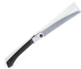
Hang one on your belt! Ideal for carpenters and woodworkers alike, this saw will cross cut with ease. Very sharp, very aggressive and very smooth. Also makes a great pruning saw. Tooth pitch: 4mm, blade length: 250mm, kerf: 1.5mm. Fitted with a convenient folding handle.
