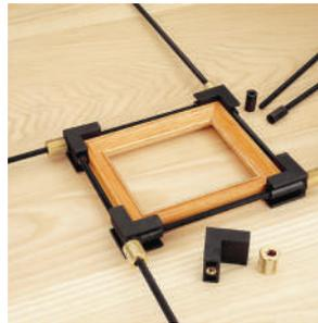
The fastest adjusting frame clamp on the market. The four clamping nuts are designed to let you make fast adjustments. They are cross-drilled to slide easily until they come up against a corner clamp, then their threads engage. To release, just back them off by a turn and they slide again. The corners are accurate extrusions with a machinists inside corner and provide a glue gullet. Kit includes extensions as shown giving a maximum capacity of 44inch square or 65inch x 23inch rectangle.
