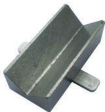
The Robert Sorby ProEdge standard gouge jig allows quick and easy sharpening and honing of standard ground gouges and carving chisels. The mitre gauge bar allows it to slide left to right so the chisel can use the width of the belt, rather than using one position only and wearing it down and generating unnecessary heat into the chisel.
