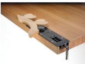
The Veritas Inset vice is a low profile clamping mechanism that is designed to sit flush in the bench, and uses the bench dogs to clamp workpieces between for a variety of different tasks. The positioning of bench dog holes being its only limitation, though the clamp travel is a massive 101mm along the 12.7mm (1/2") acme thread
