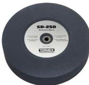
The Tormek Blackstone Silicon wheel has been designed for shaping and sharpening\* HSS and exotic alloyed steels, as well as touching up tungsten carbide. The Blackstone wheel can be graded in the same way as the Standard wheel, from 220 grit to 1000 grit. The Blackstone features sharp, yet relatively small grain, so removes hard steel efficiently even at the low speed
