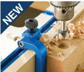
This is an ideal heavy duty stop for a router table, drill press fence, fence for radial arm saw or sliding / compound mitre saw or other tool or machine where repeatability is required that uses a fence system. The stop slides easily along the length of standard 5/16" and Universal T-tracks, securing using the 1" diameter knob.
