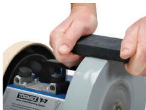
The ability to change the grit of the sharpening stone on the TORMEK T8, quickly and easily, means you do not have to reset the tool in the jig, and you do not have to go to a different grinder. This has obvious advantages. One machine, one wheel, two different grinding stages, sharpen (220 grit) and hone (approx. 1000 grit), the polish
