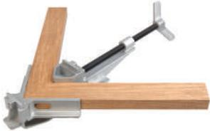
Jaws grip close to the joint avoiding bowing problems under pressure. This unit can be used bench mounted or free standing. Accepts material up to 120mm wide and 40mm thick. This clamp is ideal for joining 45 degrees mitred material at 90 degrees in applications like picture frames and carcasses.
