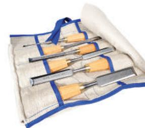
Blades are forged from K 510 steel, hardened to 60 Rc. Sides are relief-angle ground with well marked facets. Blades are finely ground and polished (blade angle 25 degrees). The Octagonal oval handles are made of strong, oiled elm wood from Switzerland and the design is very ergonomic, allowing you to shape material with ease. Available individually or in six piece set. Set
