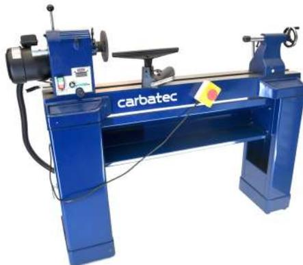
Not all lathes are created equal and this lathe has all the features to set itself apart from the pack. A heavy dust cast iron bed that is precision ground adds heft, stability and minimizes vibration. The cast iron headstock swivel through 360 deg with 45 deg and 90 deg stops for outboard turning. Perfect speeds to suit what you are turning are achieved through the electronic variable speed drive that has three speed ranges &ndash; 0 to 1000/2000 and 3750rpm.
