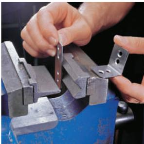
There are times when you need to bend a metal part and simply using a vice and some brute force just won't do the job. This metal bender allows anyone to form a metal part with control. The product has two parts, the male die and the V-block. Both are made of high-strength malleable cast iron that is capable of bending up to 1/8inch (3.2mm) mild steel. Each piece (about 3inch long by 1-1/8inch wide) clamps itself against a vice jaw using
