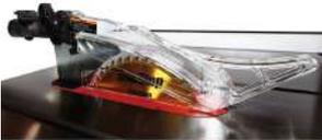
Dust collection is critical in any shop. This dust guard is collecting the saw dust right where it is being created, rather than along the entire length of the guard. This guard is standard with the Industrial and Professional models, and optional for the Contractor Saw.
