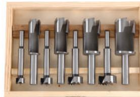
These cutters produce perfect plugs up to 50mm in length and bores the matching holes. When using barrel plug cutters the swarf should be cleared regularly by raising the drill press handle regularly, this avoids overstraining and potentially breaking the plug cutter. Drill down into the timber when cutting the plugs, but not through it, the best way then to
