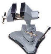
Readily attaches to any non-porous surface with a simple lever action. 76mm (3") grooved steel jaws with slide-on rubber liners. vice opens to 63mm (2-1/2") with a solid locking mechanism. Fully swivelling and tilting, it is a particularly useful vice for apartment dwellers and hobbyists.
