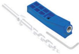
The Mini jig has the same hardened steel drill guides as the larger Kreg jigs. Its design makes it ideal for those furniture fix up jobs, by clamping, drilling and driving a screw in to complete the job. The relief hole allows waste material to escape allowing drilling to continue. It is the only Kreg jig that does not have its own fence or guide system to best position it to ensure the screws come through centrally
