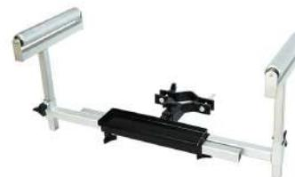
Carbatec's Drill Press Support allows larger items to be positioned safely and conveniently on the drill press, giving them support on the rollers as well as the central table. Mounts to the drill press column, and fits all models with a 60-100mm column. Two roller stand style rollers (450mm wide) are fully adjustable in height and width giving maximum versatility.
