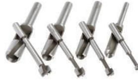
These cutters produce perfect plugs up to 50mm in length and bores the matching holes. When using barrel plug cutters the swarf should be cleared regularly by raising the drill press handle regularly, this avoids overstraining and potentially breaking the plug cutter. Drill down into the timber when cutting the plugs, but not through it, the best way then to
