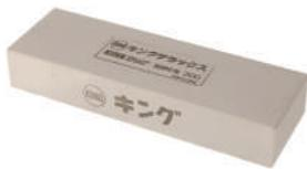
This stone is great for restoring old chisels, grinding down notches, and changing the bevel on blades. Nominal size 207 x 66mm. Note: This stone is for carbon steel blades only. For use with water only.
