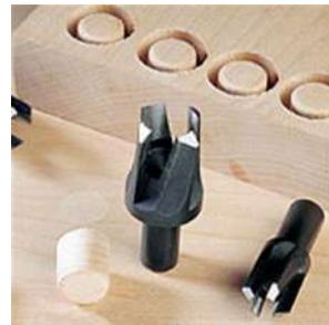
Drilling plugs to plug holes can be difficult. Drilling by hand to get an exact sized hole is not a perfect way to go, and drilling with a drill press may also not be accurate if the quill suffers from run out, therefore drilling a slightly larger hole. Tapered plugs are the solution to this problem. The first 3mm of the cutter is the stated diameter, with the rest flaring out at a 3° angle.
