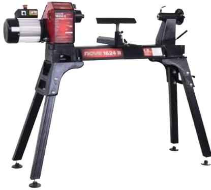
The Nova 1624-44-2 Lathe offers exceptional value for money, providing power and features that are offered only by other larger lathes. Its accessories are compatible and common between models, so if you are upgrading, all of the accessories will fit. Morse 2 tapers are fitted to both tailstock and headstock. The headstock can be rotated a full 360°, and locked where the user wants it, so outboard turning is possible, so those larger projects can be done.
