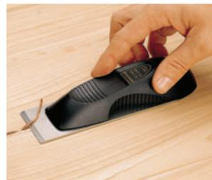
The Veritas Flush Plane features a 2" wide blade that is held in place by a 1" rare earth magnet, rather than the expected screws. This is a simple system that allows the blade to be removed and turned around so it can be stored easily or put in a pocket between uses without injury or damage.
