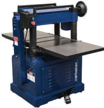
The cast iron tables on the infeed and outfeed instead of cheap rollers is just the beginning of this solid performer. Two feed rates and a rise and fall table round out the long list of features on this quality machine.
