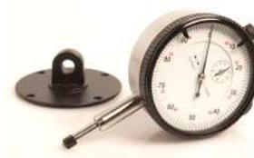
Graduated in 0.01mm with a range of 0 - 10mm. Fitted with rotating bezel with two moveable guides. Used to measure tolerances with machinery during setup. Supplied with a plastic storage case.
