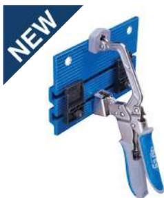
The Clamp vice combines a 3" Bench Clamp with an anodized aluminium plate that mounts to the edge of a benchtop to create a simple, highly effective bench vice. It's great for clamping pieces on edge, supported by adjustable Clamp Blocks, and for holding large pieces on top of a bench like a traditional end vice using a pair of included Bench Dogs.
