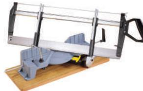
Saw carriage swings right and left 45 degrees for simple mitre cuts. Blade also tilts right and left for 45 degrees compound mitre cuts. Max. wood cutting capacity at 90 degrees: 175mm wide x 155mm high. Max. wood cutting capacity at 45 degrees left or right: 111mm wide x 155mm high. Blade length: 600mm.
