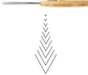
Pfeil Number. 12 chisels have a 60° V shaped profile with a straight shank, making them good for letter carving or detailed ornamentation. Swiss made Pfeil chisels come sharpened and ready for use. Regular honing is recommended to maintain the best edge for carving. They are constructed with chrome vanadium alloy that is made to Pfeil's own specifications.
