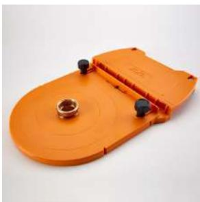
This Router Plate attaches to your BORA WTX Clamp Edge Saw Guides, providing the ability to safely and accurately route straight dadoes, rabbets and mortices, for all manner of sheet assembly work and component manufacture. Works with most routers\*\* as it comes with and utilises a standard 1" brass guide bushing to centre
