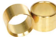
Guaranteed to never split. Chamfered on the outside at one end for handling comfort and chamfered on the inside of the other end for easy installation. Inside diameter: 22mm. Outside diameter: 25mm. Length: 17mm. Sold in pairs.
