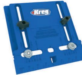
The Kreg Cabinet Hardware Jig makes drilling doors for handles that so much easier and faster. The hardened steel drill guides means the drill guides will not wear out, the edge to centre adjustment is going to cater for most desired handle positioning, and the drill guide spacing caters for standard 64mm, 96mm and 128mm handles. Clamp it to the door or drawer front
