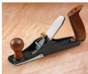
The Veritas Scrub Plane should be the tool of choice for major stock removal, and used at an angle of 30deg or more, rather than the traditionally parallel to the grain. The blade edge is ground with a 3" radius, allowing it take an aggressive cut. This is the tool needed to get stock into a condition
