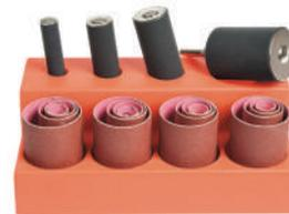
This set includes four individual drums with diameters of 1/2", 3/4", 1", and 1-1/2" respectively. Each of the drums in our "short" set are 2" in length. Set also includes 16 sleeves in total and a moulded plastic stand for the drums and sleeves as shown. Used in a drill press or lathe for contour sanding.
