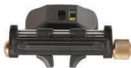
Chisels from 3mm to 38mm can be held securely in the same way the larger MK II holds blades. It will clamp bevel edged chisels up to 11.9mm (15/32") thick and square-edged chisels up to 8.7mm (11/32") thick. Narrow Blade Head ONLY - Requires to be fitted to the 05M09-01 MK11 Honing Guide.
