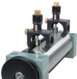
Using a pair of micro-adjustable magnets this jig will help you install new planer blades in perfect alignment with an accuracy of +/- .025mm. The easiest and most efficient way to reset your blades. Fits most planer blades. Maximum diameter of cutterhead: 130mm. Sold in a box set of two.
