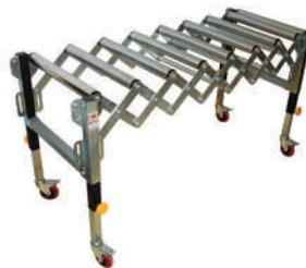
This conveyor makes movement of large workpieces easy. Simply connect the conveyor to the machine or workpiece area you'll be using it with, extend the bed to the required length and set the brakes. Next, adjust the height to meet the entry point required for your workpieces and you're ready to go. Assembly adjusts from 450mm
