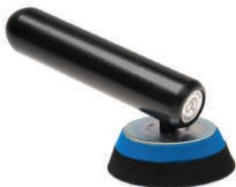
This sander has a handle made from hard plastic making it light, durable, and affordable. Attached to this is a foam backed sanding pad mounted on ball bearings. These spin freely with just enough give to conform to the inside of bowls. Supplied standard
