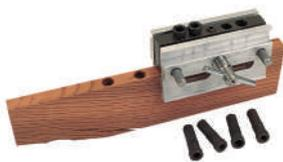
Designed for face frames or other applications where you are drilling two holes. This design has removable bushings that allow you to drill two holes of the same size without moving the jig. The holes are on 19mm (3/4") centre and the bushings and centre section are made of hardened drill
