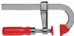
Opening 100mm, Throat 50mm. Features include: Clamping force up to 1,500 N, Step-over clamping, Comes with two plastic pressure caps, Small and easy to handle, Light weight.
