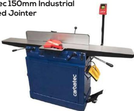
The Carbatec 6" Industrial Long Bed Jointer features an extended bed length and larger cabinet support providing trueness and accuracy without taking up too much space in your shop.
