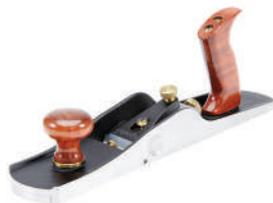
The Veritas low-angle jack plane is ideal for shooting miters, working end grain, and initial smoothing. We have designated it as a 62-1/2 because of its generous size and weight, low center of gravity, and radically set-back mouth. This is a bevel-up plane, with a 12° bed angle similar to a low-angle block plane.
