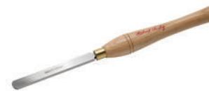
This round nose scraper has a smooth curve, so there are no corners to dig in, making this good for convex and concave surfaces. Ideal for bowls, platters and spindles.
