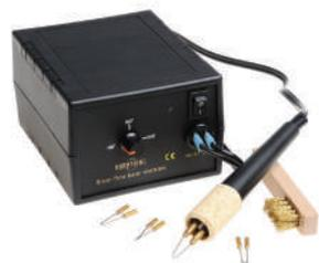
Stepless electronic unit with constant temperature control infinitely variable between approximately 350 degrees C and 800 degrees C. 230 volt; 30 watts. Powerful enough for shading. Suitable for use on wood, cork and leather. Set includes transformer, hand piece, four tips, wire tip cleaning brush, instruction book and pattern book.
