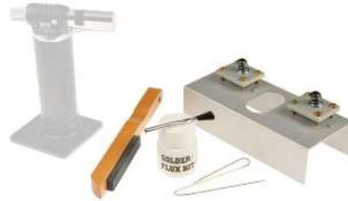
Forms brazed joints that are stronger than the base metal of the original blade, for blade widths of 1.6 to 31.75mm. This tool is used to repair broken bandsaw blades quickly, easily and inexpensively. Kit includes: brazing jig, flux, brush, silver alloy, instruction manual. A separate butane torch is required to use this kit.
