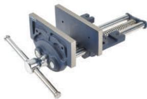
Manufactured from close-grained grey cast iron for long, trouble-free service. Its accurately machined housing assures a smooth sliding action. Accurately fitted solid steel guide rods reduce wear and tear, giving this vice a smooth and true parallel action, free of side or cross deflection. Its jaws are equipped with a "toe-in" feature. When fully closed the jaws meet only at the
