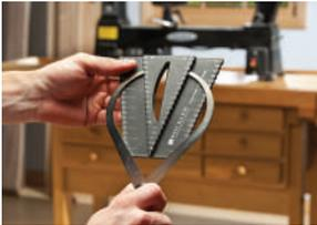
This centre finder quickly sets callipers to any 1/8" increment between 0" and 5". Also featuring a "V" shape on the back and vertical line to cut-out to easily mark the centre line on material that is round or square. The gauge is constructed of durable plastic, with easy to see white markings.
