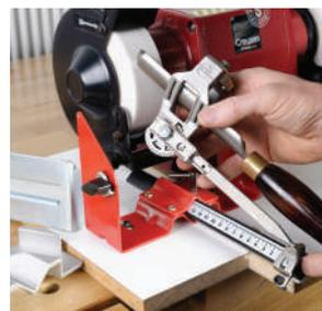
This unit features an extruded aluminium base with quick cam lock release via a comfortable rubber handle. The same finger jig as on the Nova Sharpening Centre is used; with the same tru-track ball, lightweight but strong design. Finger grinding unit combines with stationary grinding stand, resulting in a high efficiency grinding tool with minimal tool wear.
