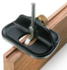
When doing woodworking with traditional woodworking tools, the Veritas router plane should be one of those tools first selected. It should be the tool used when doing stopped or through dados and grooves, and blind dovetails or for any work that requires an area cut to a precise depth.
