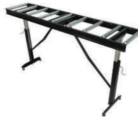
Nine rollers allow the easy transfer of long boards or panel product around the shop. The height of the stand is adjustable from 670mm to 1100mm and easily folds up for storage. Both posts are tapered so locking is positive and strong. Stand rated to 227kg. Additional rollers are available if needed. Overall length of roller stand 1670mm.
