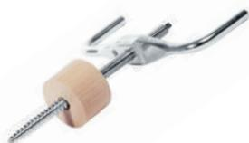
Made from Nickel plated steel. Three sizes of carvers screws are available: 155mm, 240mm, or 280mm spindle lengths. Simply drill a hole into your carving blank; and screw spigot into it through a hole in your carving bench or use with carving supports.
