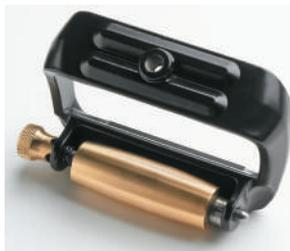
The Veritas MK.II Honing Guide camber roller allows blades to be sharpened with a slight convex curve to them, therefore avoiding the plane tracks that would otherwise occur. The barrel shape to the roller is minimal, and still gives the same support as the standard roller. Normal blade registration is used with this roller in the same way as for the standard roller.
