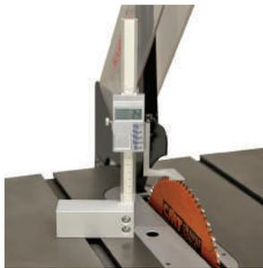
This height gauge features a digital screen read-out with readings in metric, imperial and fractional imperial. Simply zero it on your table, then slide the arm to the top of your blade or router bit etc for an extremely accurate height reading. The generously oversized magnetic base gives great stability while the L-shaped contact provides
