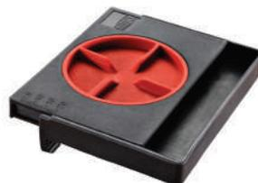
Quickly and infinitely adjustable for wall distances of 5 to 20 mm. Spacer for floating laminate and parquet flooring installations. Wide contact and support area for avoiding pressure points on the floorboards and plaster. Easy to remove by simply turning back. Very light and compact.
