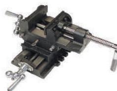
With a travel of 135mm left to right, and 160mm front to back, this is the ideal vice to use on a drill press for accurate drilling. Positive positioning in two coordinates lets you move the piece accurately. These controls provide precise adjustment for a myriad of drilling and cutting applications. Jaw width: 103mm. Maximum opening: 95mm.
