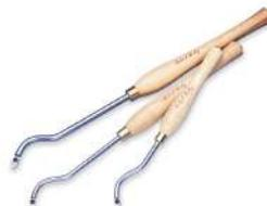
This tool can reach those hard to reach areas of turned vases that have a small aperture, or area that a straight chisel cannot reach. The 20" version has been designed for use on end grain on shallow to medium projects. The 24" version is produced from a substantial section steel, making it more suitable for both end grain and side grain working.
