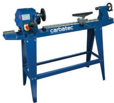
Perfect for the beginning or budget-conscious woodturner. The speed is variable via a split pulley system that allows the spindle to run between 500 to 2000 rpm. While the motor is running, turn the handle, allowing the pulleys to separate giving a different belt ratio, therefore changing the speed of the spindle. This is done easily and is an economical way to produce variable speed.
