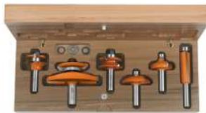
These 6 piece sets are ideal to give that professional look to your kitchen or other cabinet projects. Sets include: Perfectly matched Rail and Stile bits; Raised Panel Bit with back-cutter for milling both the front and the back on the panel in a single cut; Super-Duty Flush Trim; Ogee Style Door Edge bit and a Drawer Front bit that makes a mini raised panel cut on the outside edges of your drawer fronts. Everything required for cabinets!
