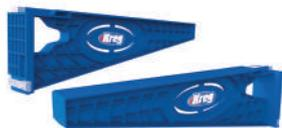
This versatile jig does it all, Kreg have done it again. The Kreg Drawer Slide Jig is going to take away all of the guess work for installing drawer slides. It is that third hand that you wish you had when doing this job. Simply mark the carcass where the runner is to go, position the jig to the mark, put the runner on the jig, and use both hands then to drive the screws in while to jig
