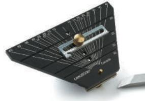
The Veritas Skew Registration Jig locks into the MK.II Honing Guide to make quick work of setting both skew and bevel angles (left- or right-hand) of chisel and plane blades. The jig's machined aluminium base provides skew angle markings that are laser etched for accuracy and legibility.
