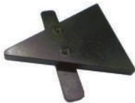
The Robert Sorby ProEdge skew jig is angled to a degree to grind and hone skew chisels. The mitre gauge bar allows it to slide left to right so the chisel can use the width of the belt, rather than using one position only and wearing it down and generating unnecessary heat into the chisel.
