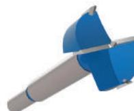
Concealed hinge boring made easy. The Kreg Concealed Hinge Bit is a 35mm Forstner style drill bit for drill flat bottomed holes for concealed hinges. These hinges are commonly used in kitchen cabinetry, so the hinge is not seen when the door is closed. The tungsten carbide cutting tips and faces give long lasting edges and a clean cut, with no tear out. The shank of the bit is designed to fit directly to
