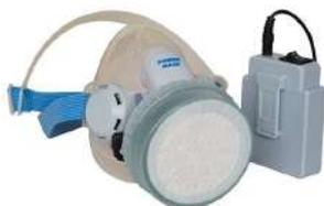
This affordable powered dust (SA-201) mask removes minute wood dust and composite particles down to 0.4 microns in size. The face cup is made of soft silicon for maximum comfort. The filtered air supply is drawn through the pre-filter then through the main filter by way of a two speed battery powered fan that slightly pressurises the mask to minimise the possibility of
