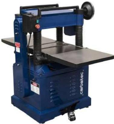
The Carbatec TH-381C thicknesser is literally stacked with features and will be a welcome addition in any workshop big or small. Features a powerful 3HP motor, a three knife cutterhead, serrated infeed roller, polyurethane outfeed roller, anti-kickback fingers, adjustable bed rollers and a front-mounted Magnetic Starter NVR switch.
