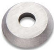
This Robert Sorby HSS internal shear scraper cutter is set to an angle of 45°, to get a good shear cut. This type of cut is less aggressive and leaves a finish that requires little to no sanding. It is an excellent choice for internal work such as goblets, bowls and other internal projects. Sharpening is done on a diamond file or honing stone, honing the top face of
