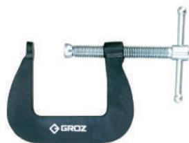
These clamps are individually forged making them amongst the strongest junior G Clamps. Frames are powder coated and Steel Screws are Zinc Plated for increased resistance to corrosion.
