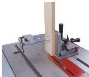
Simplifies cutting tenons and joints on your table saw. Fits most saws with a 3/8" x 3/4" mitre gauge groove and handles stock up to 3-1/4" thick. Also features 0 to 45 degrees back stop, multi-position control levers for easy adjustment and large crank handles for fast clamping.
