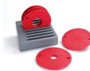
This five-piece set of Level-Loc Reducing Rings fits the Kreg Precision Router Table Insert Plate, allowing you to customize the size of the opening around the bit. The set includes rings with 3/4", 1-3/8", 1-5/8", and 2-1/8" (19mm, 35mm, 41mm and 54mm) openings, plus one blank ring that you can use to create your own custom sized or zero clearance ring. The set
