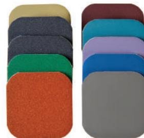
Micro-Mesh is a long lasting cloth-backed sanding product that is applied to a foam cushion layer. The paper itself is much like wet and dry paper but the addition of the cushion layer allows more control of the cutting action. While all sandpaper creates a scratch pattern, the Micro-Mesh pattern is very fine and promotes consistent sanding
