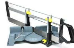
Saw carriage swings right and left 45 degrees for simple mitre cuts. Wood cutting capacity at 90 degrees: 119mm wide and 110mm high, cutting capacity at 45 degrees (right or left): 71mm wide by 110mm high. Blade length: 550mm.
