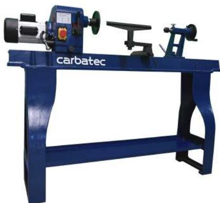
A tremendous new lathe model with all the features of a larger professional quality lathe. The speed is variable via a split pulley system that allows the spindle to run between 500 to 2000 rpm. While the motor is running, turn the handle, allowing the pulleys to separate giving a different belt ratio, therefore changing the speed of the spindle. This is done easily and is an economical way to produce variable speed.
