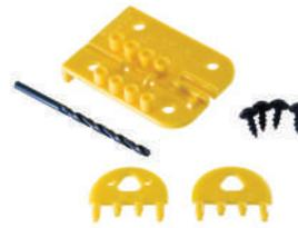
These splitters are yellow, identifying them for thin kerf blades, 2.29mm to 3.0mm. Used by woodworkers around the world, the MicroJig Splitters are positioned so one is in the same plane as one side of the blade, and the other is in the same plane as the other side of the blade. The splitters are tapered, so will not bind on the timber as it is being cut. When cutting some timber,
