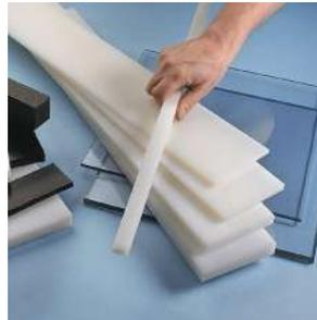
UHMW polyethylene is the material you find in most factory-made jigs. The letters stand for ultra-high molecular weight, a type of plastic that is dense, tough, rigid, impervious to moisture and, most important, has a very low coefficient of friction. Jig bases made from it slide easily on machine tables. We offer it in a range of sizes so that you can use it for making fences, jigsaw sub-tables, etc., as well as jig
