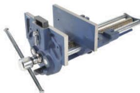
A traditional pattern woodworking vice equipped with a quick release mechanism. A simple press of the trigger initiates the quick release action, allowing the front jaw to slide freely. This allows you to interchange small and large workpieces quickly and smoothly. Then, releasing the trigger returns the mechanism to normal for
