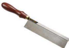
Japanese Razor Saw. 160mm blade length with 0.3mm kerf and 44TPI. Perfect for tenoning or other precision cuts.
