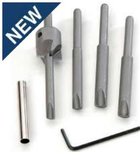
An important step in pen making requires the brass tube and pen blank to be milled perfectly square, and just as important, all glue residue should be removed from the tube before proceeding. The Universal Barrel Trimmer is by far the easiest way to do this. This set contains 4 pilot shafts to suit most pen kits and tubes, plus a heavy cutter head for squaring the blank.
