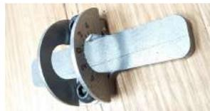
Used to hold the texturing and spiraling tools steady and at a constant angle during use, and features indexing markings for repeatability.
