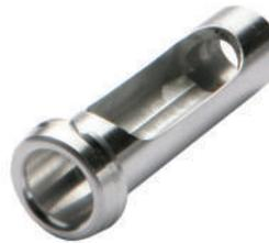
This tool has been designed to hold many of the chisels without handles. The insert takes brass tipped grub screws to securely hold the various chisels against the flat bottom of the insert. This gives the ability to use a wide variety of chisels in the longer Sovereign handle, which can also be weighted if the user desires. Using the same handle can give a familiar feel providing extra confidence to the turner.
