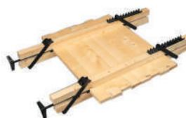
The Double Bar Clamp provides inwards clamping pressure from the ends and the face. This holds the timber together until the glue dries, and keeps the boards from moving so a nice flush result is achieved. The Double Bar Clamp requires two bars or beams general made from timber, that are a maximum dimensions of
