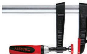
This TG series clamp has a 80mm throat and is fitted with plastic caps. Threading in the sliding arm engages serrations in the rail when the sliding arm is inclined, ensuring maximum security and restricting slippage. These versatile clamps are a must when you
