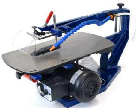
A high performance, low-vibration scroll saw with many features and benefits that will be prized by the serious scroll saw user. This scroll saw delivers those features and will be appreciated by the more discerning scroll saw user. The stroke rate is continually variable, allowing almost any material to be cut (with the right blade fitted). The 20mm deep stroke allows deeper sections of timber to be cut, clean and square.
