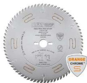
Ideal for cutting ply, and cross-cutting timber, this blade features CMT's general purpose chrome coating and laser cut noise reduction slots. The coating protects the blade from overheating, prevents corrosion and rust, minimises resin build-ups, improves chip ejection and improves performance and cutting life.
